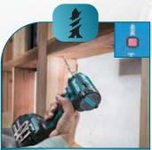
The tool drives a screw with low-speed rotation at first. After starting to impact, the rotation speed increases and reaches max speed.
