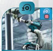
This mode helps to prevent a bolt from falling off.
