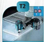
Driving self-drilling screws to a thick metal plate with good finish.
