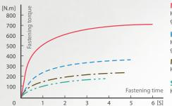
Max mode (4) High strength friction grip bolt M24
