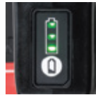
Battery fuel gauge
