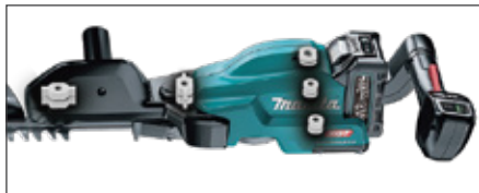
Anti-vibration structure consisting of Motor-crank section and handle section linked by cushions to absorb vibration from blade and motor-crank section
