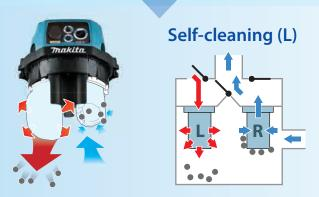
2) About 10 seconds after, the vacuum air flow toward one of the two filter units is automatically reversed by air flow control valves engaged with a DC motor powered cam, then the air blast forcibly expands compressed Damper to shake off dust from the Prefilter while the vacuum operation continues using the other filter unit.
