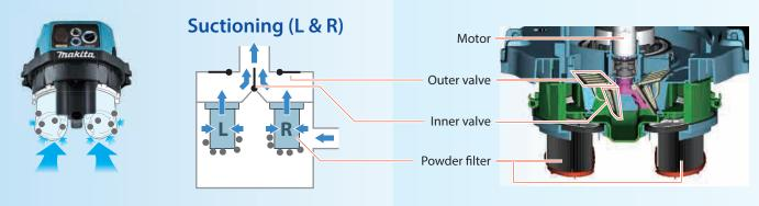
When switched on, the machine starts vacuum operation using two filter units, and each Prefilter of the two filter units collapses into itself to compress Damper, and fits closely over Damper and Powder filter.
