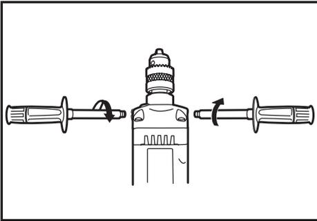
Screw the side grip on the tool barrel securely. The side grip can be installed on either side of the tool, whichever is convenient.
