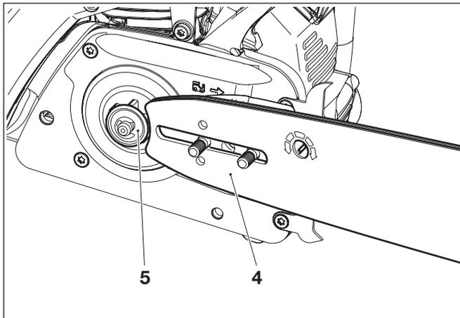
Put the guide bar (4) on and push it against the sprocket (5).
