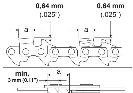
The sharpening angle ( $\alpha$ ) must be identical for all cutters!
