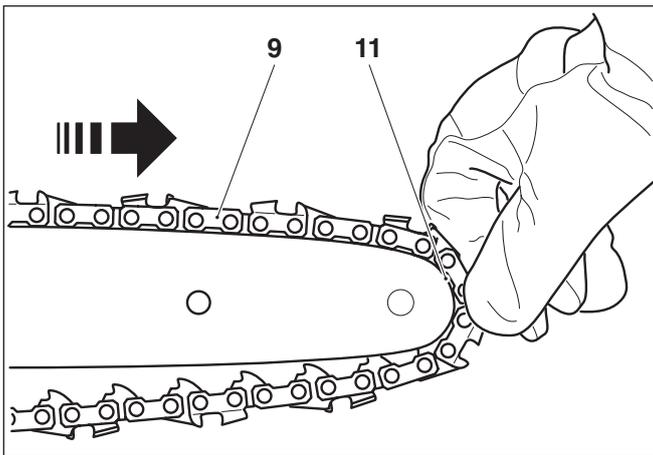
Pull the chain (9) around the sprocket nose (11) of the guide bar in the direction of the arrow.
