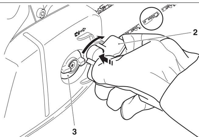
Release the sprocket guard chain tensioner until it turns freely, then fold it in between protective ribs (15) as shown in the illustration.
