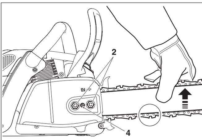
**Tightening the saw chain**
