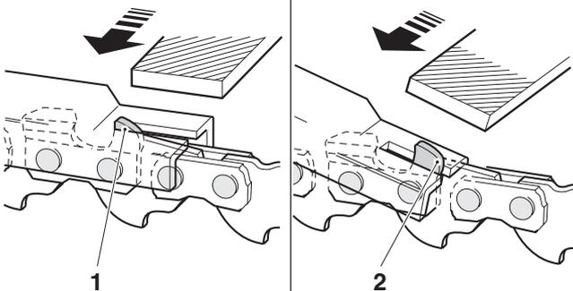
After having sharpened the chain, the height of the depth limiter must be checked by means of a chain gauge.
