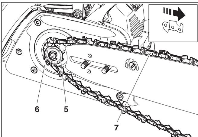
Lift the chain (6) over the sprocket (5).
