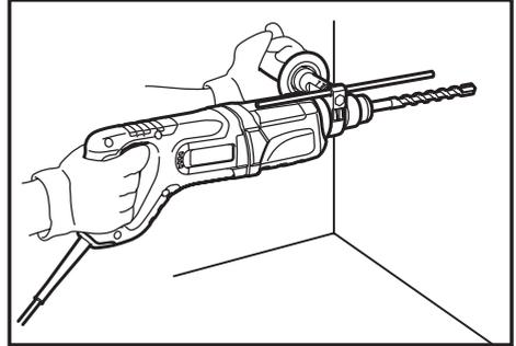
Set the action mode changing knob to the
