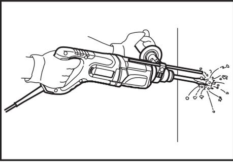
Set the action mode changing knob to the
