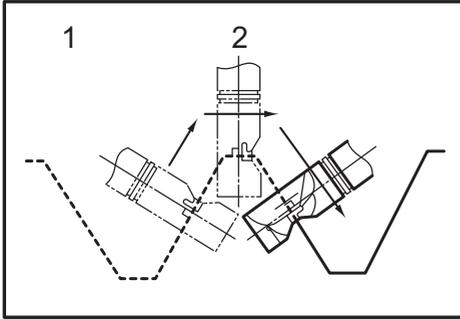
► 1. From the side view 2. Cutting head should be at right angle (90°) to cutting surface.
