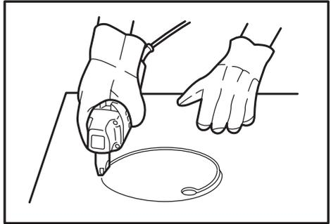
Cutouts can be done by first opening a round hole over 21 mm in diameter which the cutting head can be inserted into.
