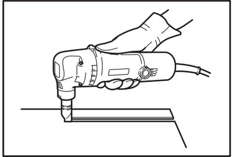
Hold the tool so that the cutting head is at a right angle (90°) to the workpiece being cut. Move the tool gently in the cutting direction.
