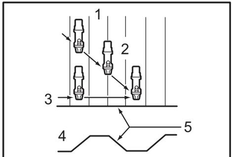
► 1. From the top view 2. Cutting at an angle to grooves 3. Cutting perpendicular to grooves 4. From the side view 5. Corrugated or trapezoidal sheet metal
