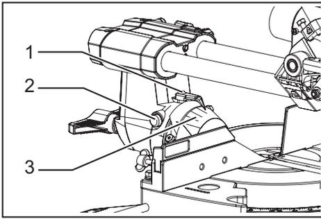
► 1. Pointer 2. Release button 3. Bevel scale
