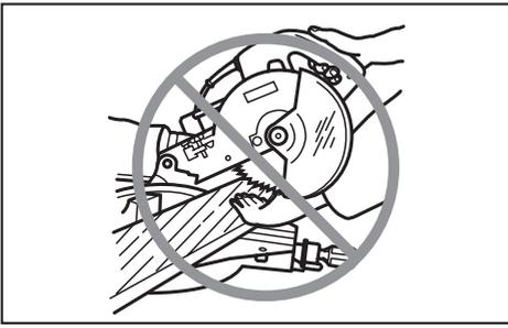
6. **Do not reach behind the fence with either hand closer than 100 mm from either side of the saw blade, to remove wood scraps, or for any other reason while the blade is spinning.** The proximity of the spinning saw blade to your hand may not be obvious and you may be seriously injured.
