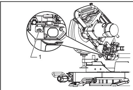
► 1. Screw holding the laser unit box
