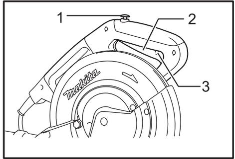
► 1. Lock-off button 2. Switch trigger 3. Hole for padlock
