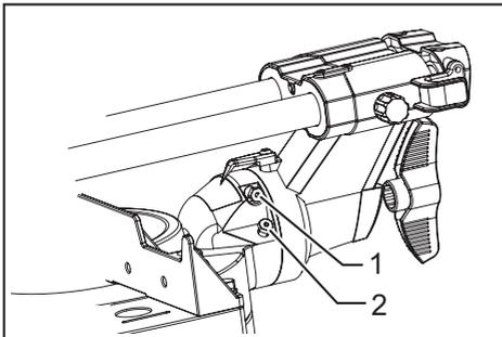
► 1. 0° adjusting bolt 2. Left 45° bevel angle adjusting bolt
