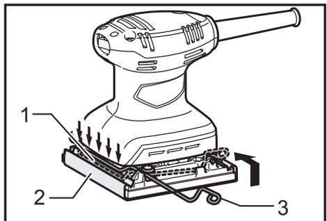
► 1. Clamping part 2. Abrasive paper 3. Lever
