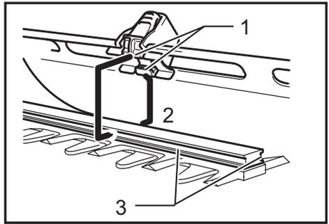
► 1. Hooks 2. Fit the hooks into groove 3. Grooves
