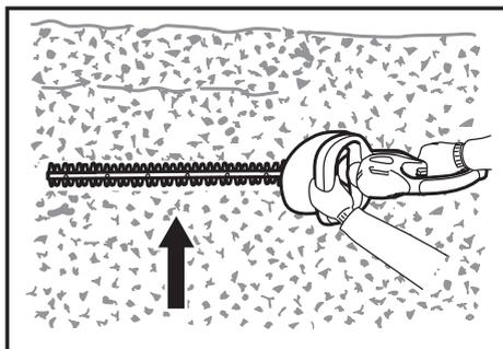
Cut upwards with both hands pull the switch triggers B and C and move it in front of your body.
